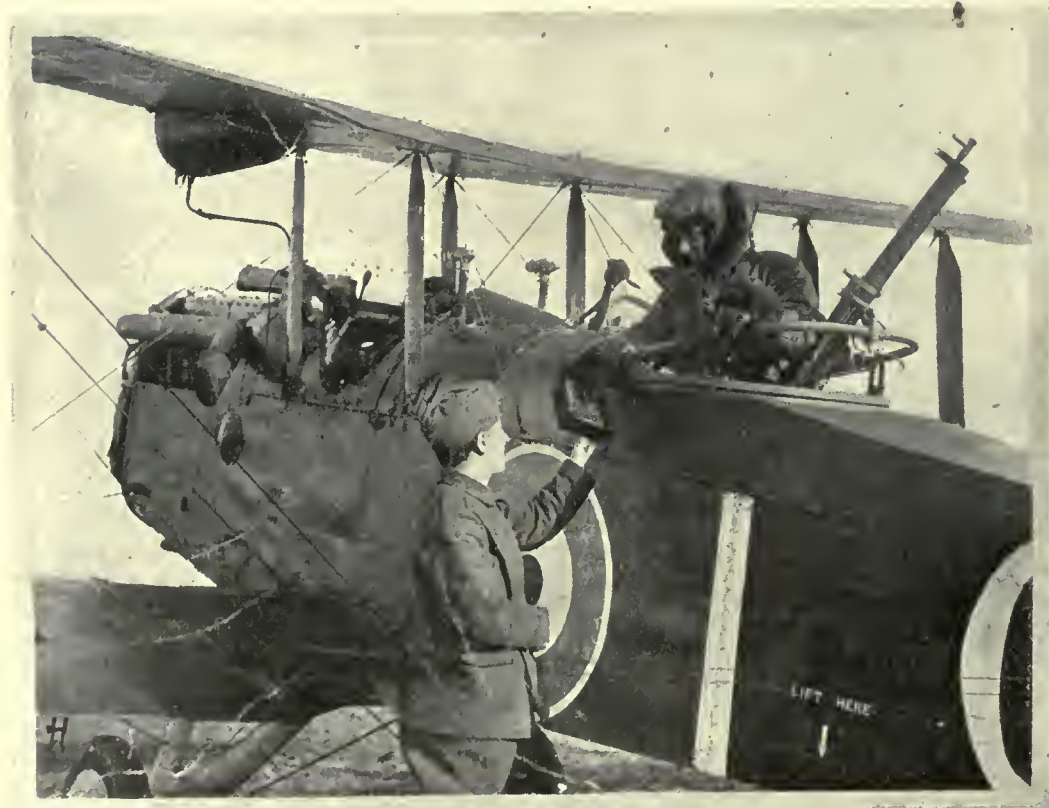
AERIAL PHOTOGRAPHY: HANDING PLATE SLIDES TO A PHOTOGRAPHER IN A BOMBING MACHINE.
